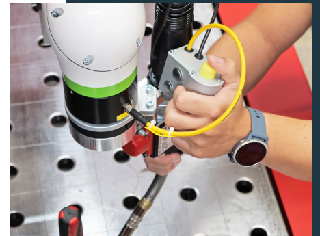
Simple welding path programming due to direct torch guidance
